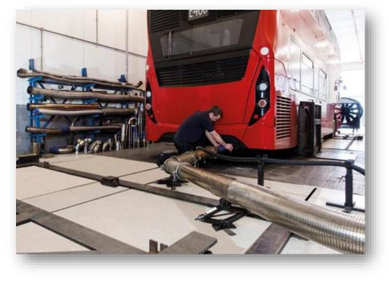
Millbrook's Variable Temperature Emissions Chamber (VTEC) is a climatic chassis dyno vehicle emissions testing facility designed for light and heavy duty vehicles.
