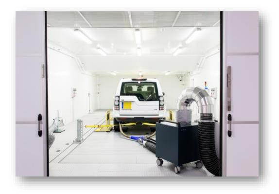
Millbrook's 4WD climatic emissions chassis dynamometer operates at temperatures between -20°C and +50°C
