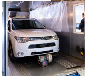
VTSHED (Variable Temperature Sealed Housing for Evaporative Determination)
