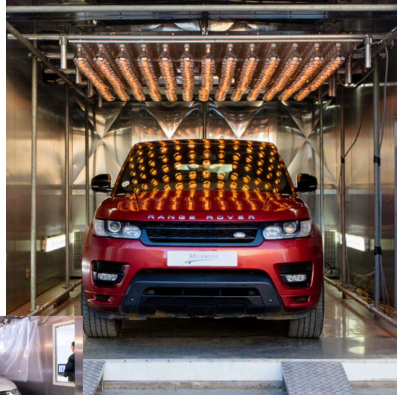
VTSHED (Variable Temperature Sealed Housing for Evaporative Determination)
