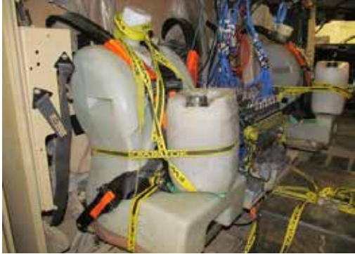
Fig 1: The troop compartment of an MoD Ridgback ballasted and instrumented for legislative whole body vibration, hand arm vibration and workplace noise data gathering.
