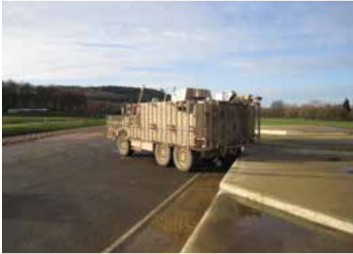
Fig 1: An MoD Mastiff 2 reverses up the 500mm Step Climb to assess its mobility and usability
