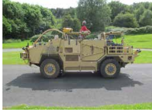
Fig 2: An MoD Jackal ballasted and instrumented for legislative whole body vibration, hand arm vibration and workplace noise data gathering, note the Anthropomorphic Test Device (ATD) in the gunner's position.
